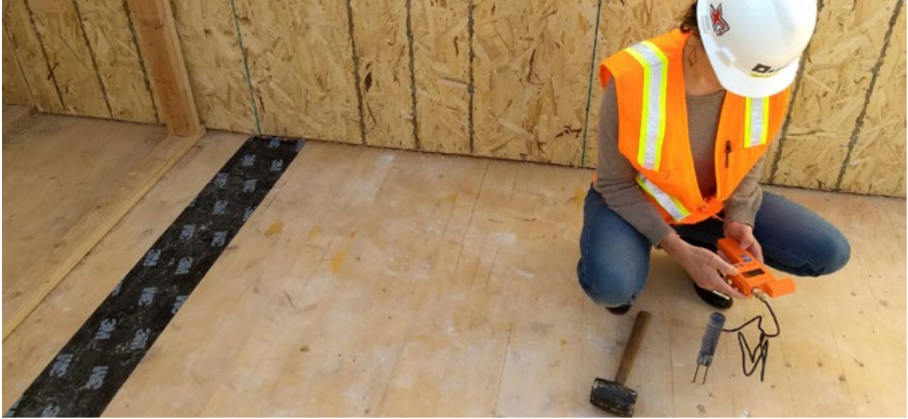
FIGURE 5.22: MOISTURE MONITORING CLT FLOORS WITH A HAMMER-IN PROBE
