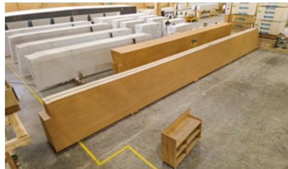
TOP: V-SHAPE GLULAM BEAMS STRUCTURALLY GLUED AND SANDED PRIOR TO SEALER APPLICATION
