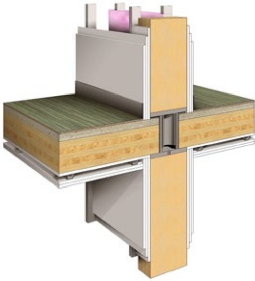
FIGURE 5.23: END-GRAIN TO END-GRAIN COLUMN CONNECTIONS MINIMIZE SHRINKAGE
