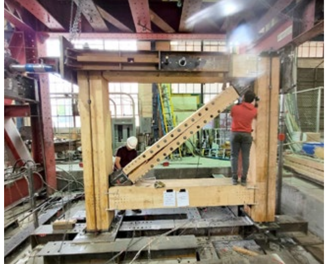
FIGURE 5.18: TIMBER BRB FRAME TEST Source: Timberlabs
