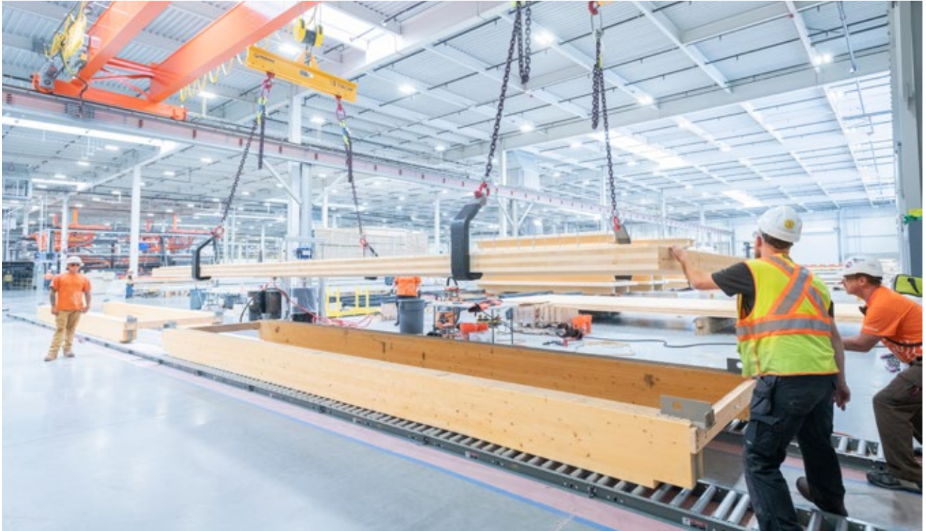
FIGURE 6.7: ASSEMBLING PREFABRICATED COMPONENTS IN A FACTORY SETTING
