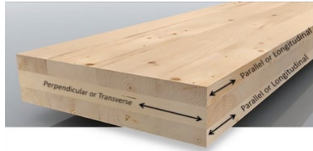
FIGURE 3.1: ILLUSTRATION OF A MASS TIMBER PANEL'S MAJOR (PARALLEL OR LONGITUDINAL) AND MINOR (PERPENDICULAR OR TRANSVERSE) STRENGTH DIRECTIONS
