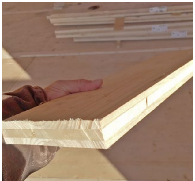
FIGURE 5.5: SPLINE CONNECTION MATERIAL EXAMPLES: PLYWOOD AND JOINERY BOARD
